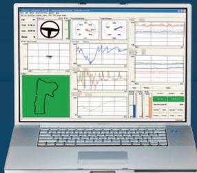
Transmitted telemetry data can also be logged on the pit computer for immediate and detailed evaluation in *i2* while the vehicle is still out on track, assisting with strategic on-the-spot decisions and well planned pitstops.
